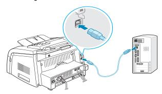
If you want to use a parallel printer cable, purchase only IEEE 1284 compliant parallel cable and connect it to the parallel connector on your machine.
